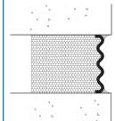
Seismic Colorseal is held in place by the backpressure of the expanding foam in conjunction with a field-installed bead of silicone caulk at the substrate-to-bellows interface.
